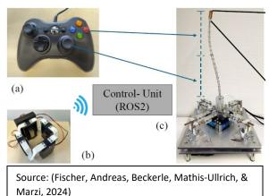
systems with non-contact localization. This comes into play in surgical procedures where visual feedback alone is not sufficient. Thus, we aim to equip a robotic arm with a capacitive sensor that communicates with a haptic feedback bracelet to guide the user through an arbitrarily shaped phantom.
